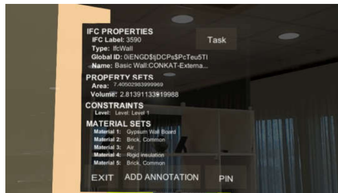
Figure 109. IFC properties menu as visualized after performing the air tap gesture on a static building component (wall) of the BIM model of the CONKAT building while the ARIBFA tool was tested on VR mode in the KRIPIS building.
