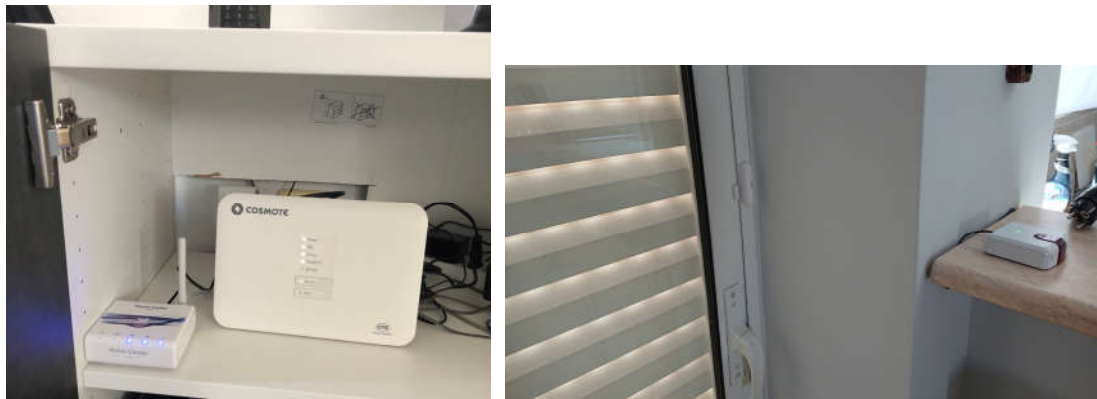
Figure 82. left) Gateway installation in CONKAT's pre-validation building, right) The sensor installed in the southeast door of the living room and the living room A/C controller
