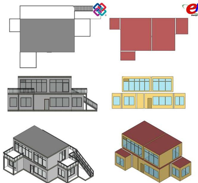
Figure 6 IDF Generator results – Rendering the generated IDF geometry in SketchUp
