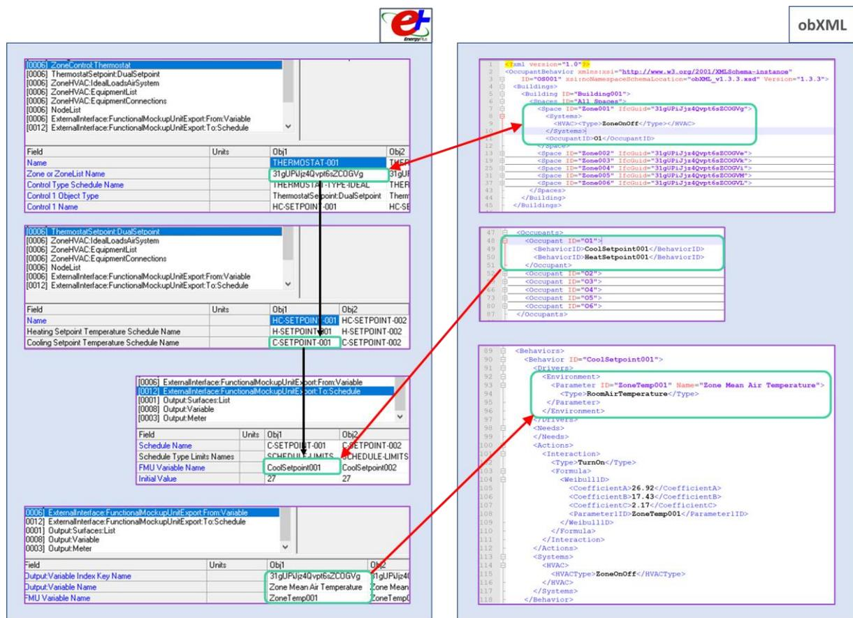
Figure 8 EnergyPlus and ObXML co-simulation: parameters setup – EnergyPlus sends the zone air temperature to and receives the thermostat cooling setpoint from the obXML at each timestep
