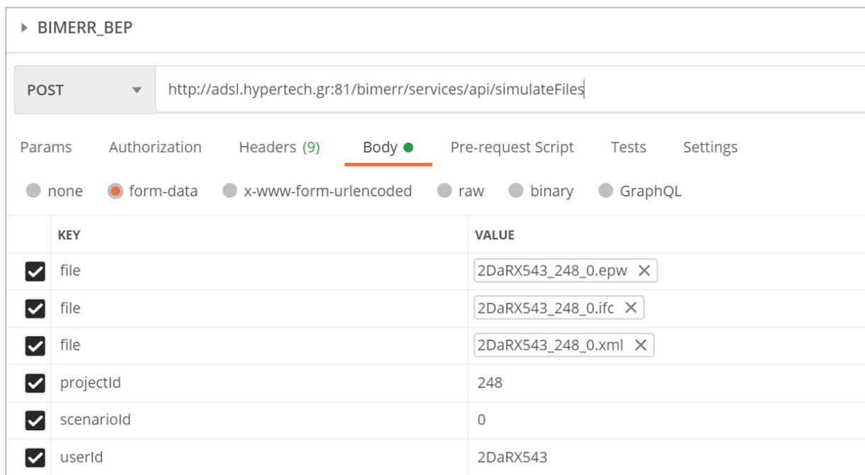
Figure 5 Postman request to the BEP module endpoint for the baseline Energy KPI calculation
