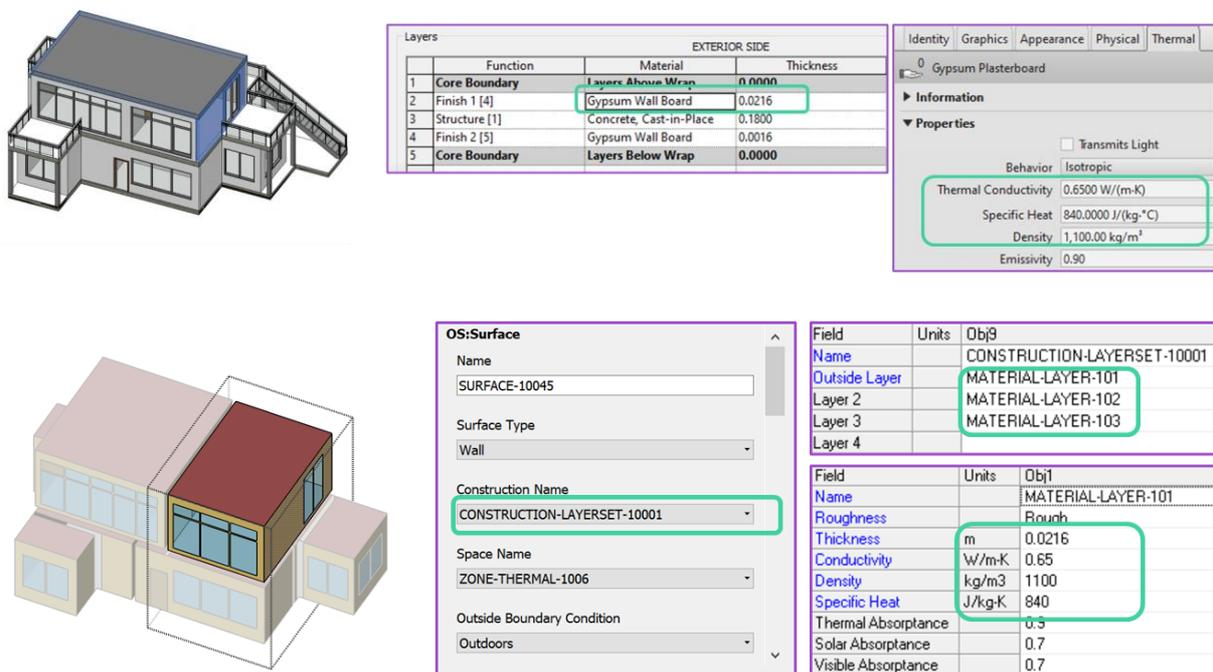
Figure 7 IDF Generator results – Construction (material layers sets) and material thermal properties
