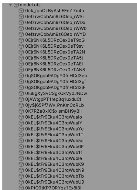
Figure 11a: Non-hierarchical structure of imported OBJ in Unity.
