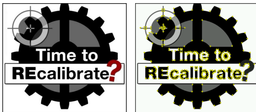
Figure 15: An image target used in the ARIBFA application and an illustration of the extracted features.
