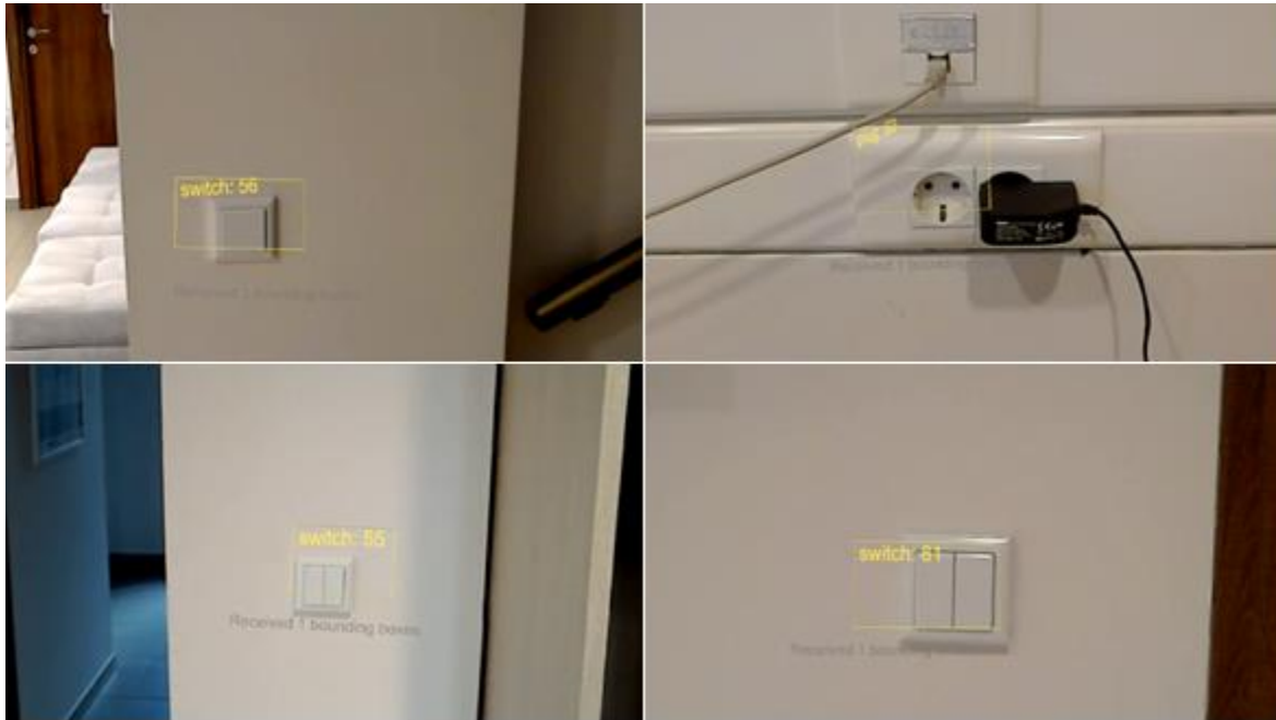
Figure 34: Images depicting detected MEP components using 2D bounding boxes in DesktopARIBFA application.
